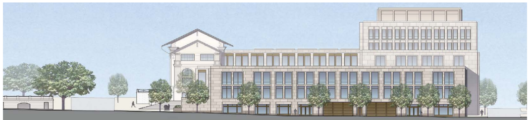
South Elevation with 3 stories to allow sunlight to penetrate the courtyard and atrium beyond
